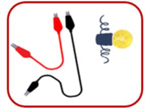
3. Connect the **Red** alligator clamp to the long arm of the LED & **Black** alligator clamp to the short arm.
