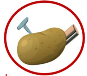
2. Attach the end of the **Red** alligator clamp to the copper (+) and the **Black** alligator clamp to the zinc nail (-).
